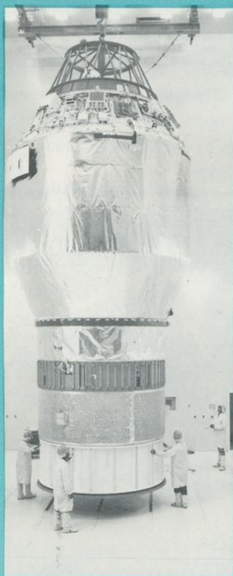
The first wide-body Centaur upper-stage vehicle for the Titan IV program is shown being positioned in a General Dynamics thermal acoustic test chamber in San Diego. General Dynamics' Space Systems Division will roll out the vehicle on Nov. 13.
