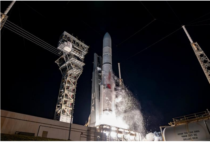
ULA's Vulcan rocket is powered by a Centaur V upper stage, which the company wants to upgrade over time to fly long-duration missions. (United Launch Alliance)
