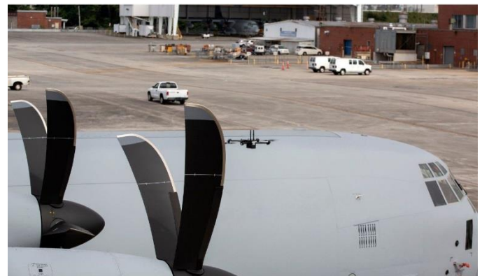
Drone inspection of a C-130J using AAIR.
