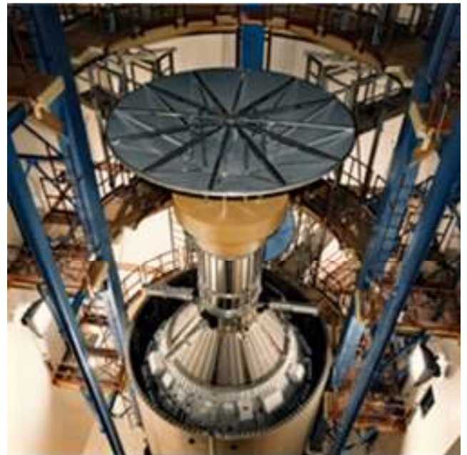
Acoustic Test of Cassini Model Photo Credit: Provided by Jason Cowley
