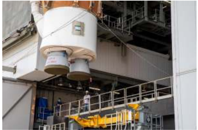
The first stage of a United Launch Alliance Atlas 5 rocket, seen here with its RD-180 engine, is lifted into position on a mobile launch platform inside ULA's Vertical Integration Facility at Cape Canaveral Air Force Station. Credit: Kim Shiflett/NASA
