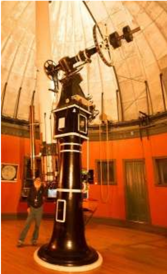
Jack at the Chamberlin Observatory 126 year old 20-inch Clark/Saegmuller refracting telescope, circa 1894
