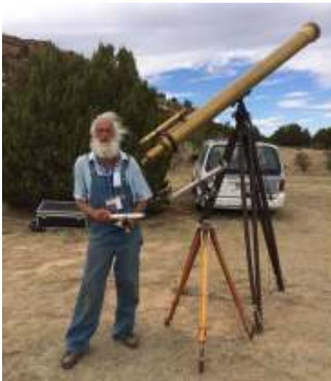
Jack at the Okie-Tex Starparty, where the skies are dark and unpolluted. The large telescope is a 6-inch refractor by Alvan Clark 7 Sons, made in 1877; the others are homemade tiny 'scopes, done just for fun. Photo: Chris Wilkerson.
