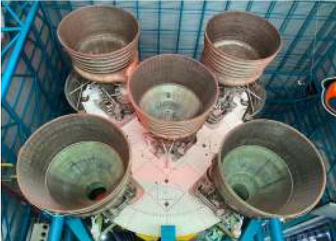
**Five Stage I F1 Engines on Restored Saturn V**
