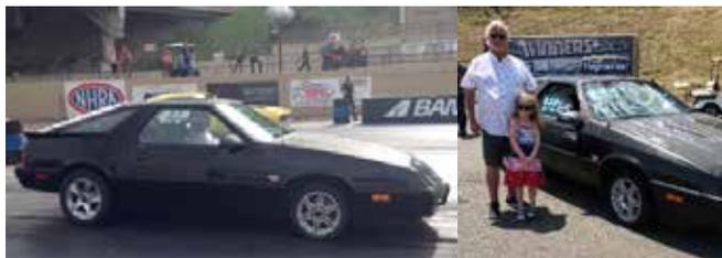
**1987 Dodge Daytona – Ran 15.3 in the 1/4 mile at 87 mph at Bandimere, Denver, CO – Dodge 2.2L Throttle Body Injection 170 hp weighing 3050 lbs. including driver**
