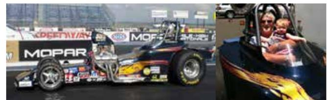
**23T Altered – Ran 7.72 in the 1/4 mile at 175 mph at Bandimere, Denver, CO – Dodge 572 Single 4 Barrel 1000 hp weighing 2100 lbs. including driver**
