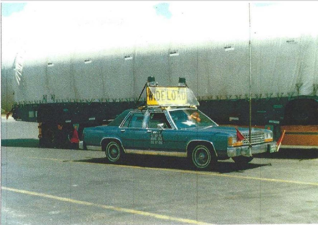
Photo #1 Shows Wide Load Sign and Tall Antenna, Lead Car Next To Stage I, Ready To Go
